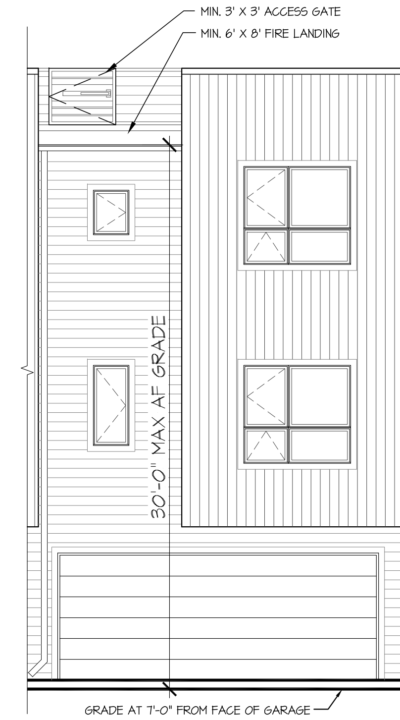
6 TYPICAL ELEVATION SCALE: 3/16" = 1'-0"
